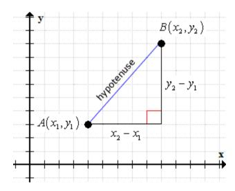
Finally, applying the concept of the Pythagorean Theorem, the distance formula is calculated as follows:
