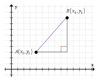
Find the legs of the right triangle by subtracting the x-values and the y-values accordingly.
