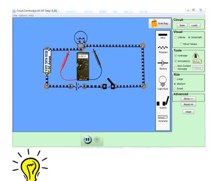
✓ It should be noted that the voltmeter measures the potential difference, so one (black electrode) must be connected to the region where the energy of the electrons has not been used up yet and the other one (red electrode) must be connected to the region where the electrons have already given up some of their energy to the bulb. That should give you a difference.
