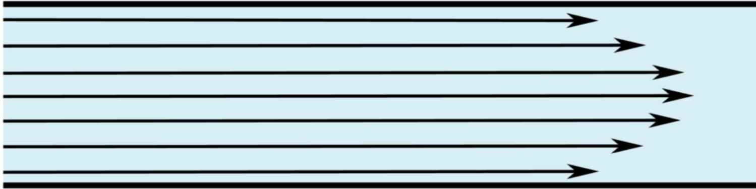
Fluid particles follow a smooth path in layers or laminae with each layer moving parallel to each other without mixing; has visible stream lines
